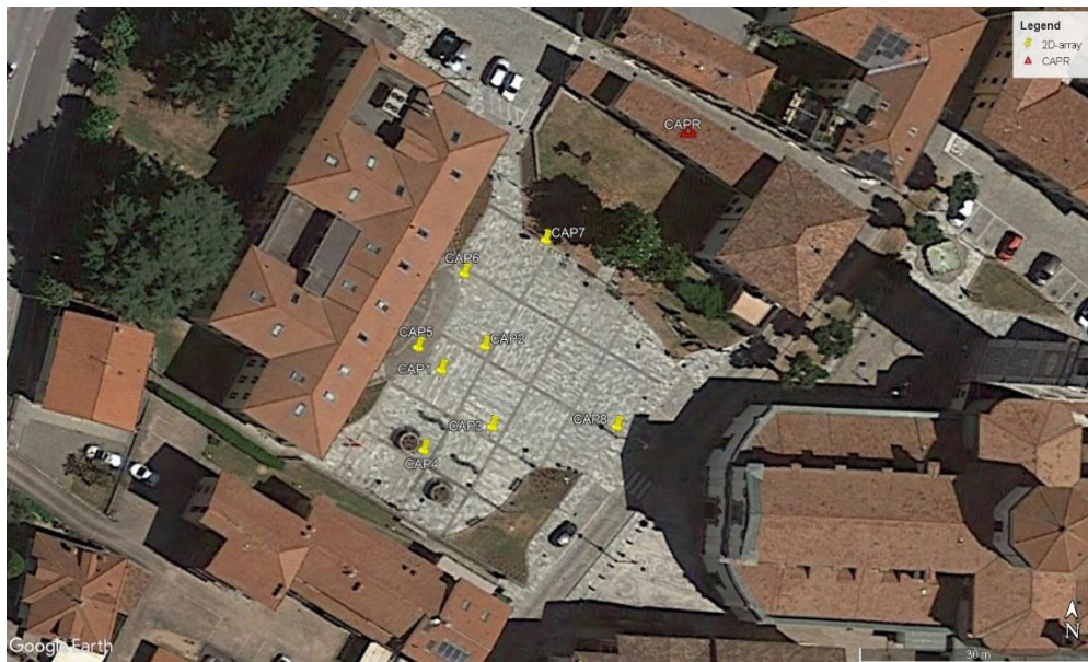
Figure 6: Map of the geophysical measurements performed at the IV.CAPR site. The yellow place-markers indicate the geometry used for 2D array in passive configuration. The red triangle indicates the IV.CAPR accelerometric station (image from Google Earth http://www.earth.google.com ).
