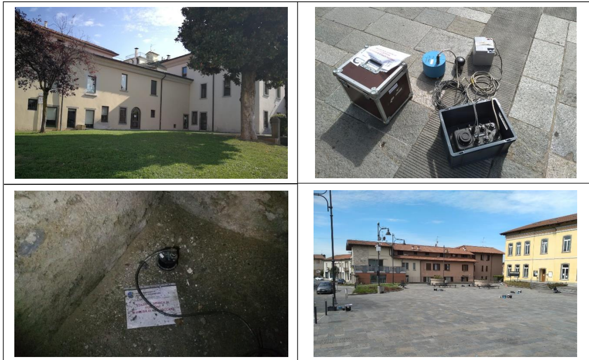
Figure 7: Upper left: library where the IV.CAPR accelerometric station is installed at Capriolo (BS). Bottom left: IV.CAPR accelerometric station. Upper right: single station ambient noise measurement. Bottom right: 2D passive ambient noise array installed close to the IV.CAPR station.
