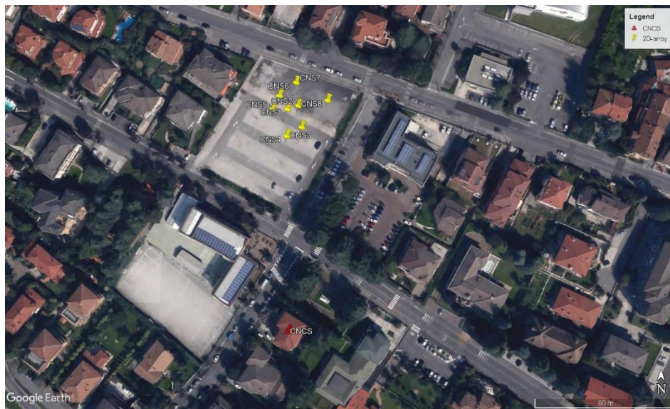
Figure 6: Map of the geophysical measurements performed at the IV.CNCS site. The yellow place-markers indicate the geometry used for 2D array in passive configuration. The red triangle indicates the IV.CNCS accelerometric station (image from Google Earth http://www.earth.google.com ).
