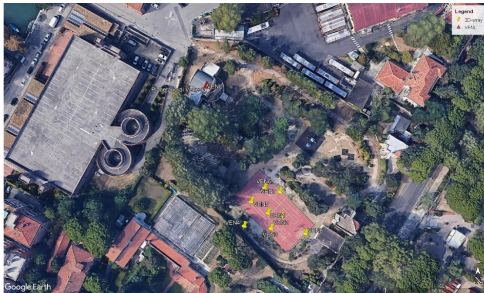
Figure 6: Map of the geophysical measurements performed at the IV.VENL site. The yellow place-markers indicate the geometry used for 2D array in passive configuration. The red triangle indicates the IV.VENL accelerometric station (image from Google Earth http://www.earth.google.com ).
