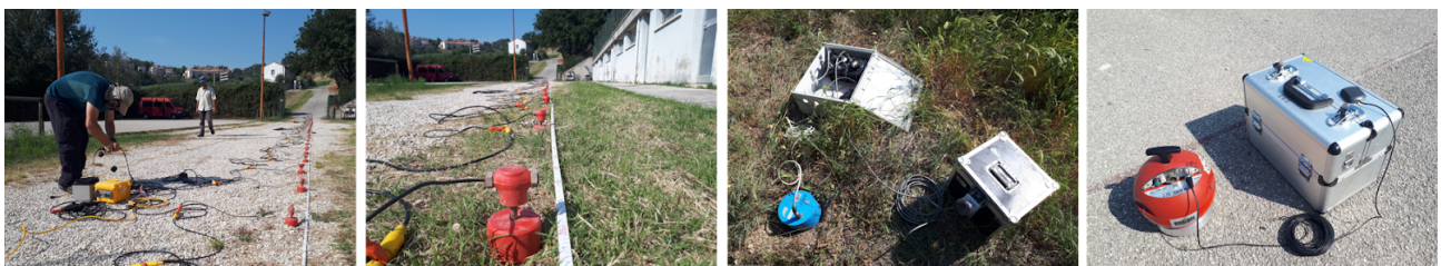
Figure 4. Deployment of MASW line and seismic stations. The last two pictures show the TR01 station (Lennartz 5s velocimeter with a Reftek130 digitizer) and the TB03 station (Terrabot).
