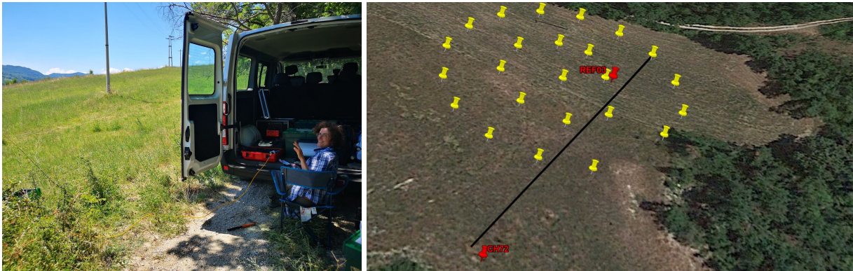
Figure 10: On the left a picture of the field where the 2D passive array was set, on the right a map with the geometry. The yellow markers indicate the 24 vertical geophones (eigenfrequency 4.5 Hz). The red markers show single-station noise measurement (REF03 and CH72 discussed before). The black line indicates the position of the linear active array (71 m long) performed about 2 weeks later (6th of September 2019).
