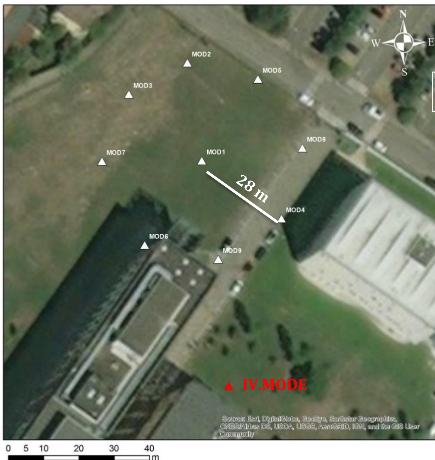
Figure 1: Map of the geophysical measurements performed at IV.MODE site. The white triangles are the nine stations of the 2D array in passive configuration (all stations are equipped with Reftek-130 digitizer and Lennartz 3D-5sec velocimetric sensors). The red triangle indicates station IV.MODE.
